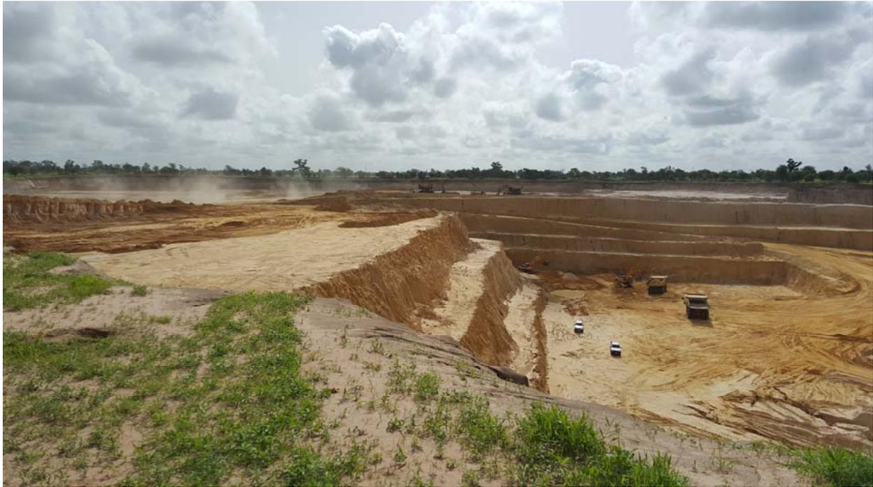
*Figure 3: Stage 1 open pit to the right of picture showing phosphate mining operations, with overburden stripping of Stage 2 open pit in the background to the left of picture.*
