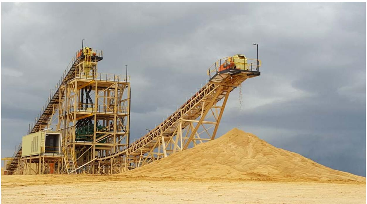
*Figure 2: First production at the Wet Screening Plant with power generating plant to the left of picture.*
