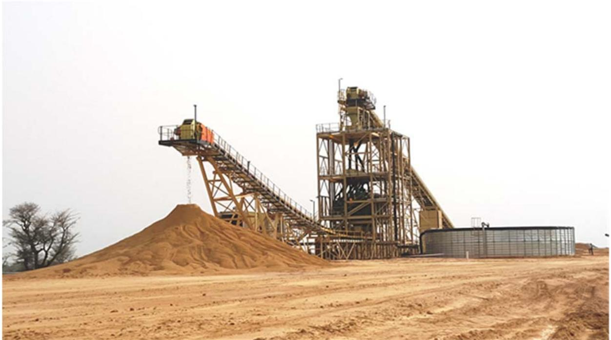
*Figure 1: First product being discharged off of the Product Discharge Conveyor at the Wet Screening facility,*
