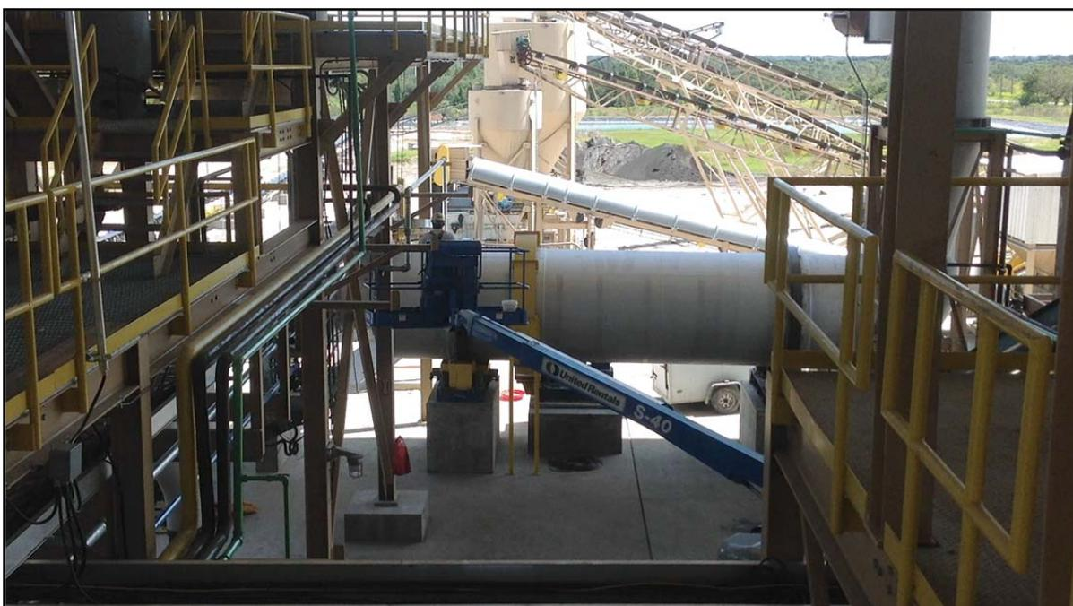
Figure 3: View of the feed drier at the JDCP Demonstration Plant
